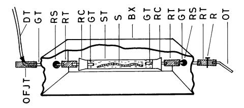
Figure 2. Position of specimen tube inside the box. BX, box; DT, discharge tube; GT, glass tube; OFJT, outlet from finger joint tube; OT, outlet tube; R, regulator; RC, rubber cork; RS, rubber seal; RT, rubber tube; S, specimen (earthworm); ST, specimen tube.
